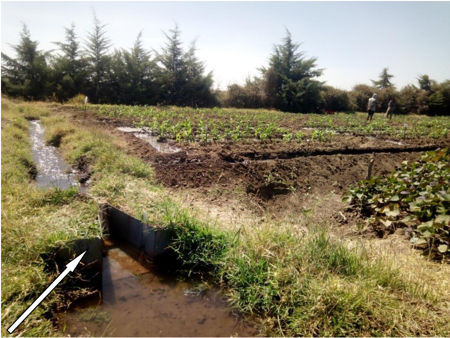
Appendix figure 2: Discharge measuring Parshal flume
