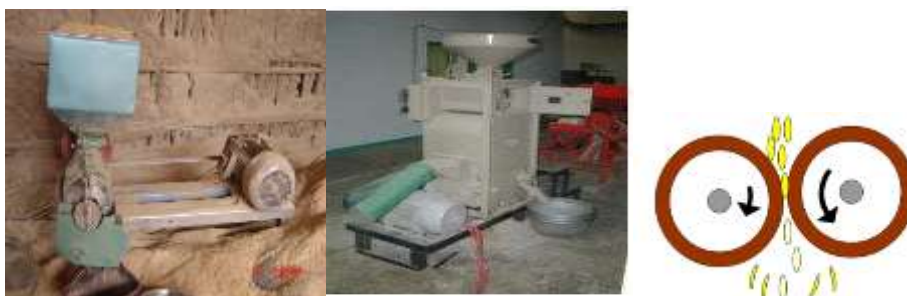
Figure. 2. Single pass Engelberg rice mill (left), double pass SB10 rice mill with rubber rollers for hulling(middle and right) commonly available in rice producing areas of Ethiopia
