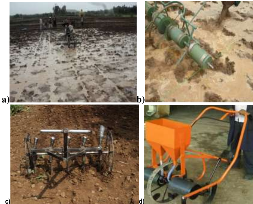
Figure 3. a) & b) Hand pulled 8 row IRRI seeder under testing by the Bahirdar Mechanization & Food Science Research c) 5 row upland rice seeder development by the then Bahirdar Mechanization and Food science Research d) IRRI modified seeder by EIAR. Photo sources: a), b) & c) by Mr. Abu Tefera & d) by Mr. Yonas Lema (Yonas L, 2014)
