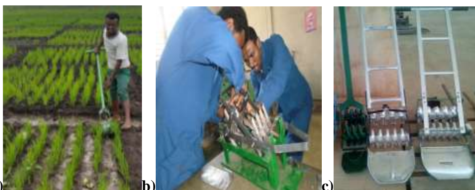
Figure 7. a) Hand pusher rotary weeder under testing at Fogera NRRTC, b) Construction of the rotary weeder by researchers in Madagascar c) Rotary weeder for paddy imported from Japan for demonstration.
