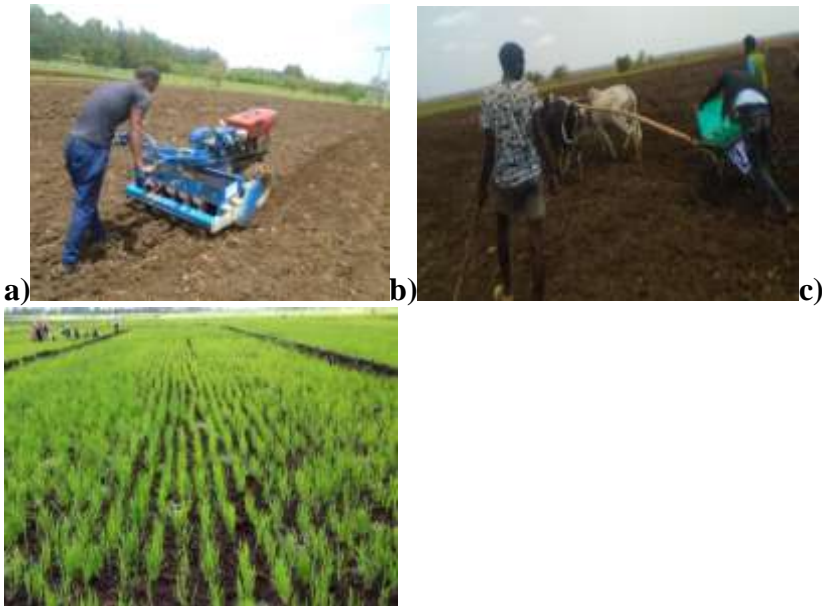
Figure 4. a) On station evaluation of 2BFG seeder b) 4 row oxen drawn upland seeder developed by EIAR c) Rice field seeded by the 2BFG seeder.
