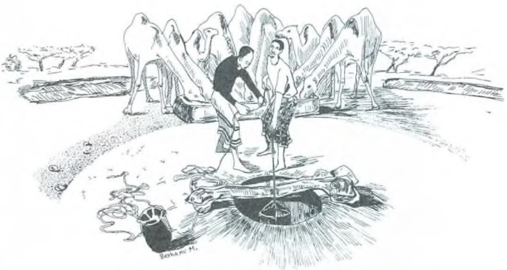
This riverbed well has a concrete apron and is lined to keep the water clean
