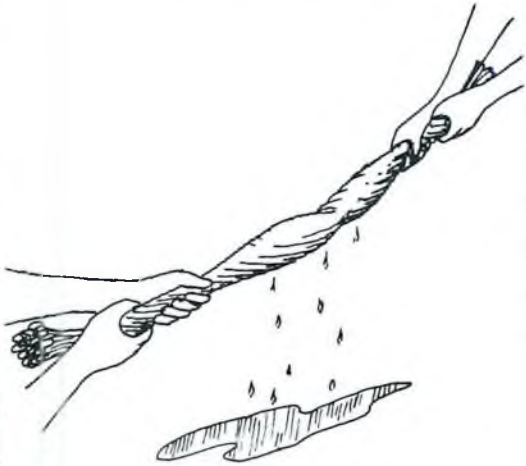
Fig. 23: Squeezing through fiber band wringing in Wolayta
