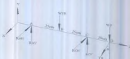
Figure 6. Forces acting on fan shaft and their locations.
