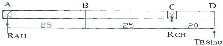
Figure 9. Free body diagram of fan shaft on horizontal (XZ) plane.
