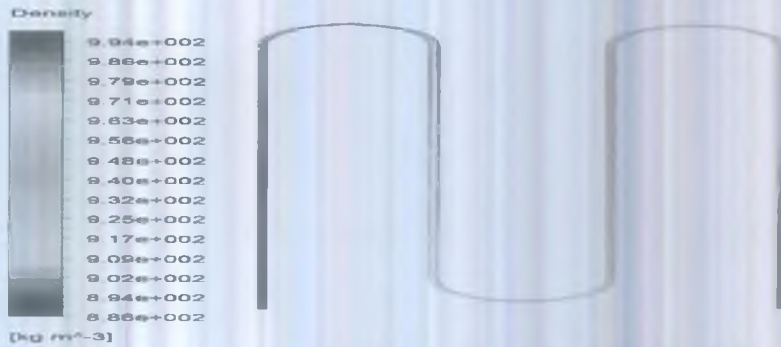
Figure 7. Density contours of water in serpentine tube
